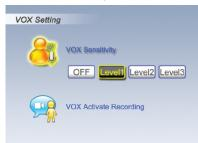
Allows user to set the level of sensitivity for voice activated recording. Level 3 is the highest sensitivity level. This system setting will be set and applies to all cameras while recording.
