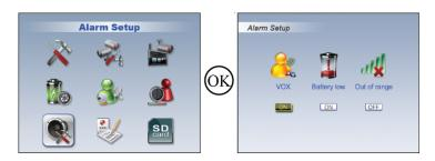
Press W to shift to ON/OFF. Press  $\blacktriangleleft$   $\blacktriangleright$  to move between items.
