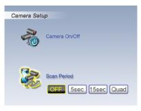
Use  $\blacktriangleleft$  b to change Scan Time interval from OFF / 5 sec / 15 sec / Quad, press W to confirm the settings.
