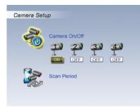
Use  $\blacktriangleleft$  b to select the camera (selected camera highlighted in black.) Press R to change ON/OFF status.
