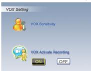
System will auto record for 30 sec once camera is triggered by voice when "VOX Activate Recording" is set to ON.
