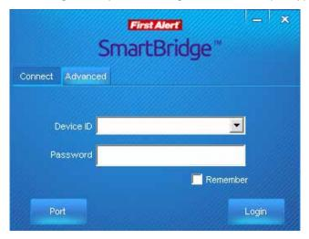
Click Port to enter the port settings. This is to assign a router port that is open. Typically, this is set to 9101 (recommended)
