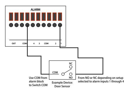
Note: Switch COM must be connected to COM in alarm block for device to operate properly
