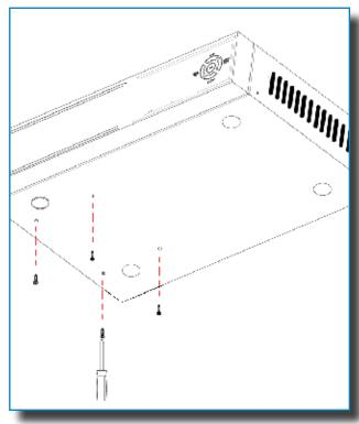
Hard Drive Remove/Install Screws from Below
