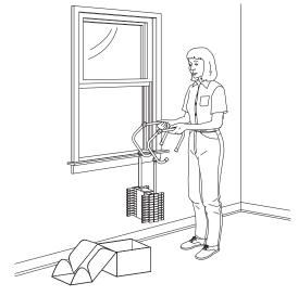
3. Place the sill hooks firmly over the windowsill and pull the release strap to deploy the ladder.
