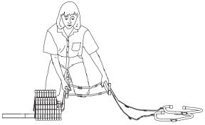
4. Use the plastic strap (attached to the bottom rung) to wrap and secure both layers of rungs. This will minimize the chance of the ladder becoming tangled when you remove it from the box in an emergency.
