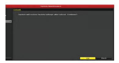
(NOTE:) All NVR parameters will revert to the default settings excluding the network parameters: IP address, subnet mask, gateway, MTU, NIC working mode, default route, and server port.
