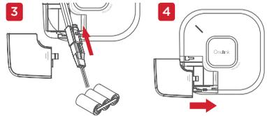
If the alarm does not test, check the battery to ensure it is properly connected and the alarm is properly mounted in the bracket.
