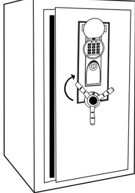
Rotate handle clockwise, then pull door open
