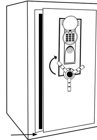
Insert key and turn counterclockwise and hold. Rotate handle clockwise then pull door open.
