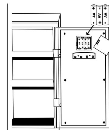
Install 4 "AA" batteries in the correct direction
