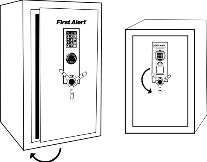
Push door closed then rotate handle counterclockwise fully into the locked position.
