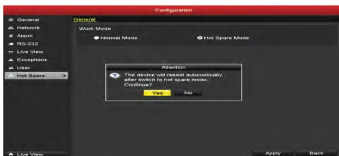
**NOTE:** The camera connection will be disabled when the device works in hot spare mode. It's highly recommended to restore the defaults of the device after switching the working mode of the hot spare device to normal mode to ensure the normal operation afterwards.
