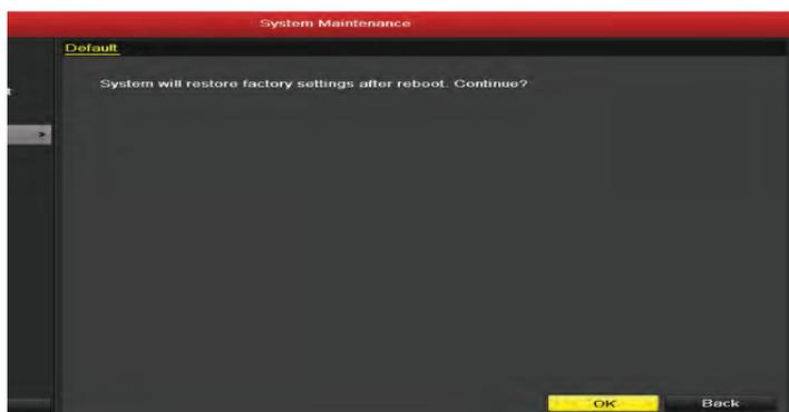
The screenshot shows a "System Maintenance" window with a "Default" tab selected. The main content area displays the text: "System will restore factory settings after reboot. Continue?". At the bottom right, there are two buttons: "OK" (highlighted in yellow) and "Back".
