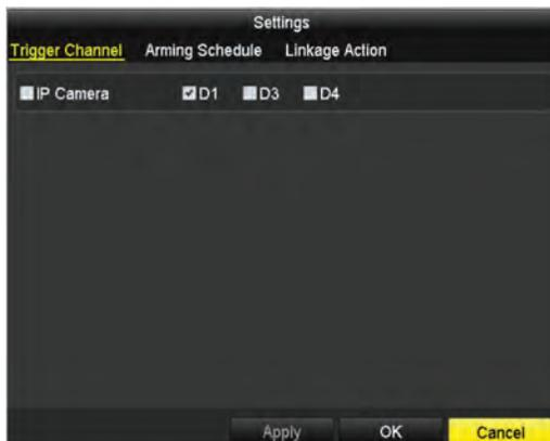
5. Select the channels which you want the motion detection event to trigger recording.
