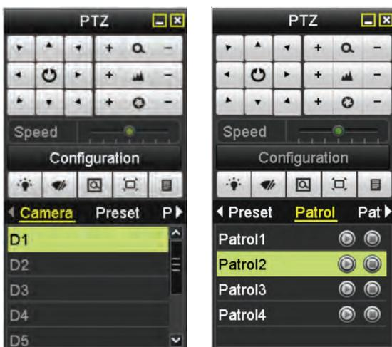
**NOTE:** In PTZ control mode, the PTZ panel will be displayed when mouse is connected. If no mouse is connected, **PTZ** icon appears in lower left corner of window, indicating that camera is in PTZ control mode.
