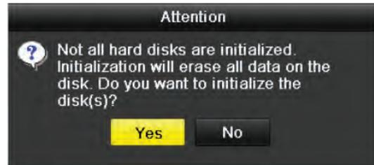
The HDD can also be initialized through the HDD Information interface: Menu > HDD > General.
