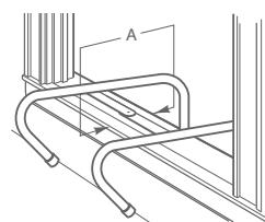
**DIMENSION A:** The windowsill width should be between a minimum of 6" (15 cm) and a maximum of 10" (25 cm).
